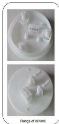
Flange of oil tank
